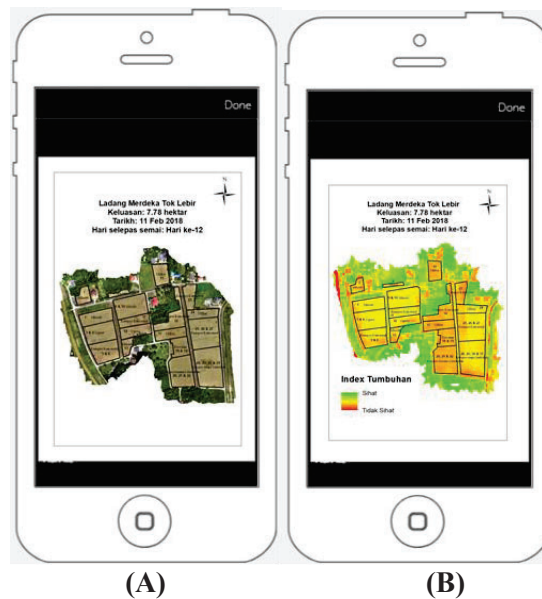
Figure 5. Example of images (A) RGB image (B) Multispectral image captured by UAV [15].
